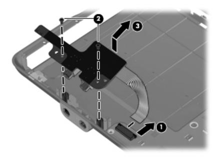
Reverse this procedure to install the audio board.
